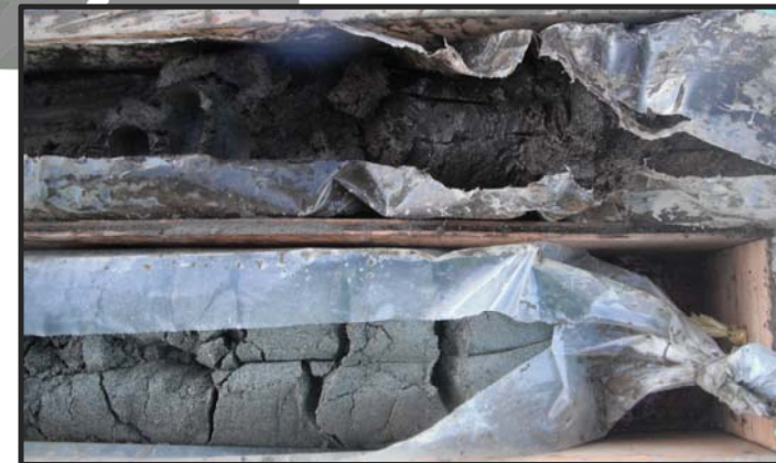
Fraser River organic silt (top) and sand channel deposit (bottom), Coquitlam
